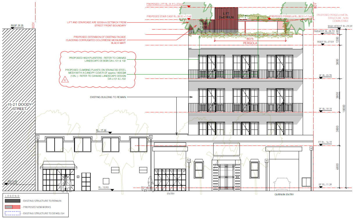
Figure 7: Proposed North Elevation Plan (Doody Street) showing the extent of the proposed works to the rooftop including lift and lift overrun, extension of fire stairs and pergola
